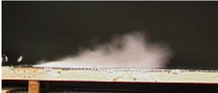
Figure 4. Corn starch dust cloud produced from air blast over dust layer (from Scherpa, 2002)
