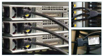
The Z-ATS™ HV Hydra versions allow a single Z-ATS™ unit to protect 2 or 3 devices from a power failure simultaneously. Please note that the total load of all served devices cannot exceed the rated load of the Z-ATS™.
